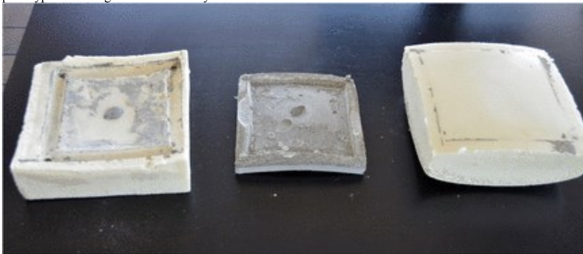
Fig. 14 The first cast (23 cm x 23cm×23 cm) prototype utilizing the new mould system. The foam mould on the left represents the negative mould, and the foam mould on the right represents the positive mould. Fig. 14 shows it was possible to create a continuous double curved surface with an edge return using the new mould system. Fig. 15 This capability to create a freeform thin-walled GFRC element with an edge return is necessary to meet the demands of current architectural applications that require a visually desirable monolithic appearance.
