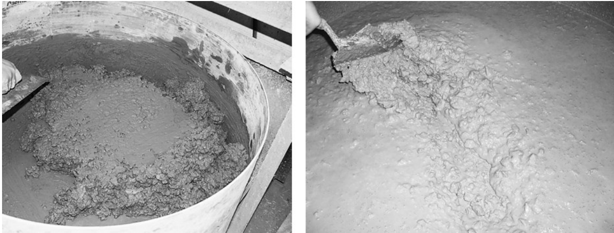
Figure 3 HLPC before and after the addition of SP
