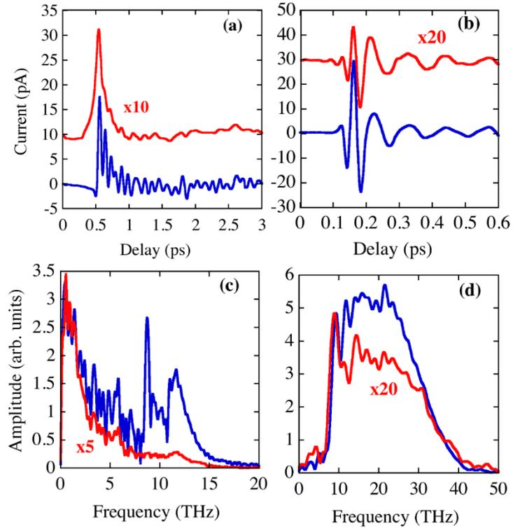
Fig. 1: (Colour online) (a), (b) Time domain signals for GaAs (lower traces) and SOX (upper) receivers obtained using InAs and a 30  $\mu\text{m}$  thick GaSe crystal at a phase matching angle of  $60^\circ$  as THz sources respectively. The traces are offset for clarity. (c), (d) are corresponding spectra (upper curves: GaAs, lower : SOX).
