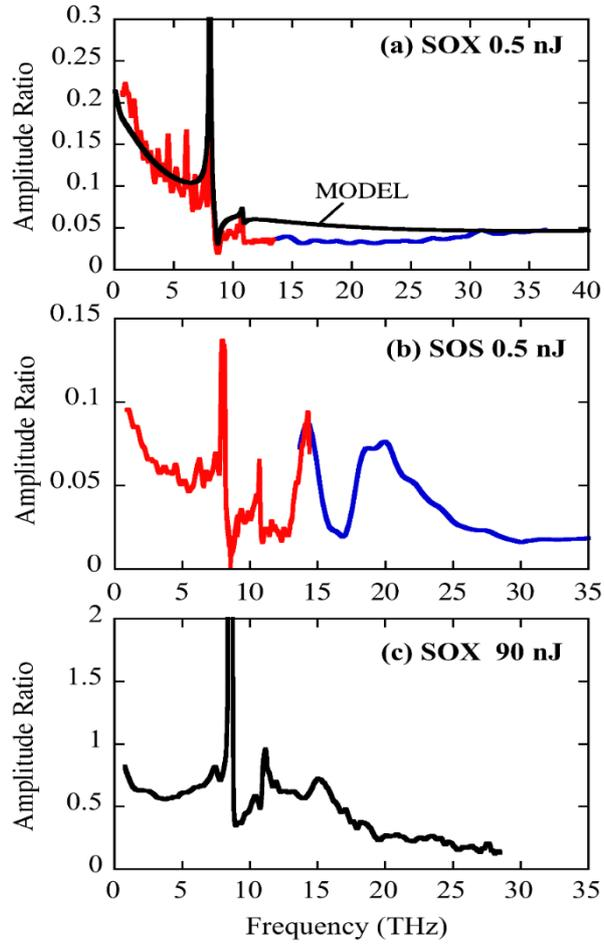
Fig. 2: (Colour online) (a), (b) Ratio of signal spectra of SOX and SOS receivers relative to that of GaAs at a sampling pulse energy of 0.5 nJ. Left hand portion (red) is obtained with InAs source, right hand (blue) with GaSe. The sharp peaks below 7 THz are due to a Fourier transform artefact. In (a) the black curve is a calculation described in the text. (c) SOX ratio at probe pulse energy of 80 nJ.
