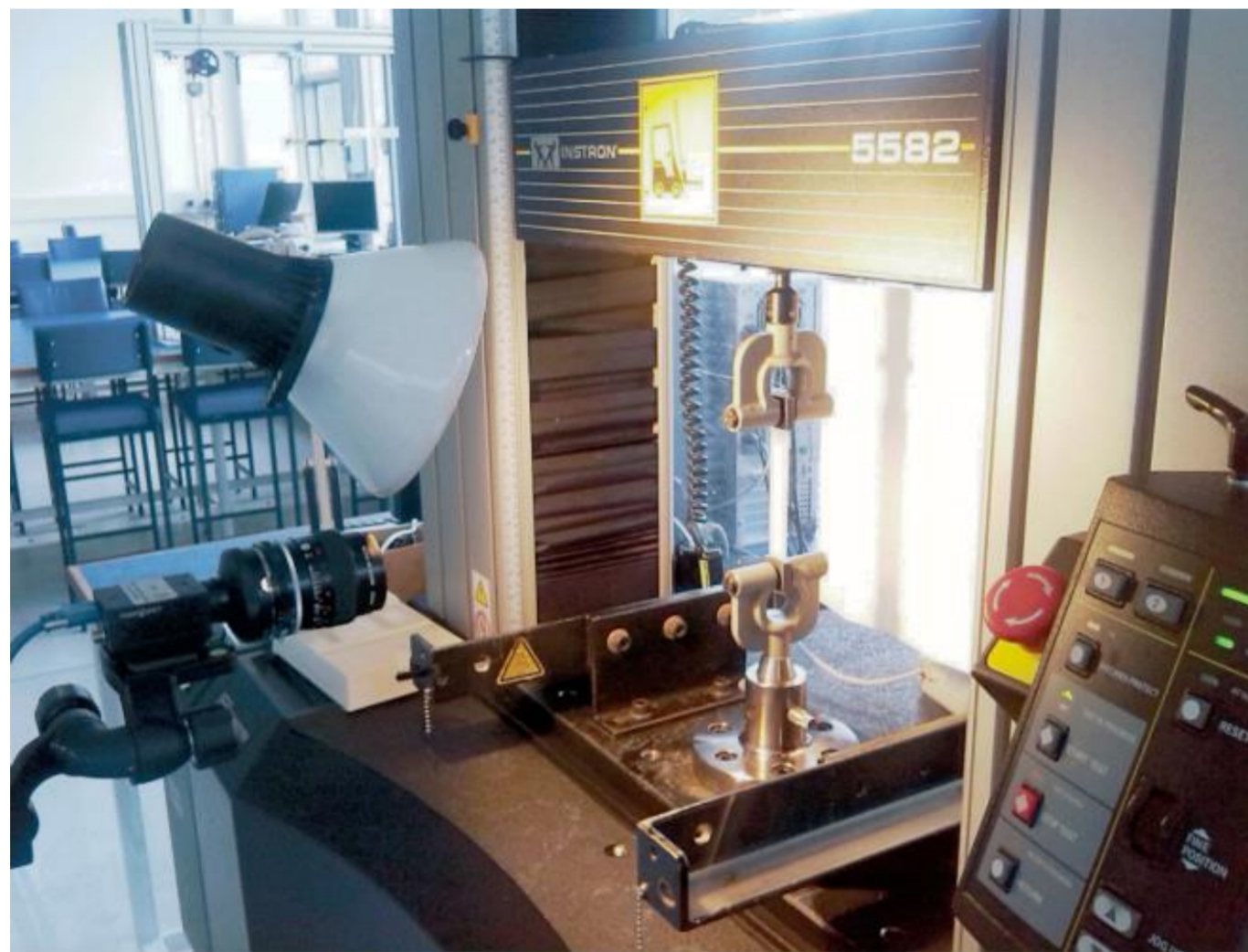
Fig 2: Viscoelastic characterisation of the UHMWPE
