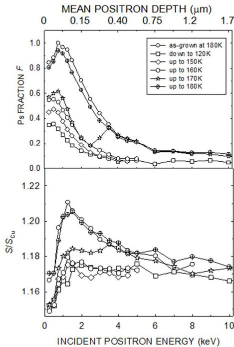
**Figure 2.**  $F(E)$  and  $S(E)$  for ice film grown at  $180\text{K}$ , measured at  $180, 170, 160, 150$  and  $120\text{K}$ . Note the jump from low to high parameter during the second  $170\text{K}$  run.
