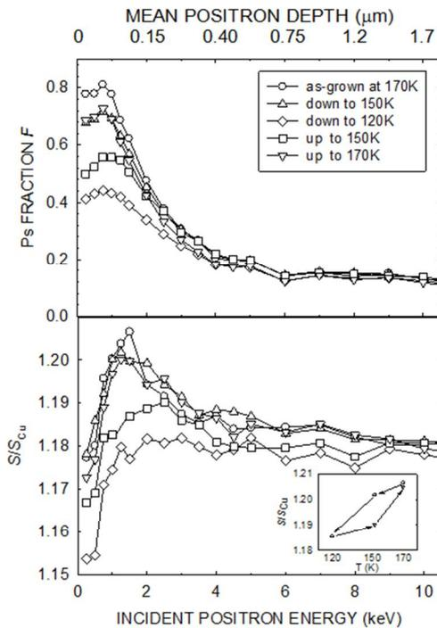
**Figure 1.** The Ps fraction  $F(E)$  and  $S(E)$  for ice film grown at  $170\text{K}$ , measured at  $170, 150$  and  $120\text{K}$ . The inset shows the hysteresis in the peak  $S$  value as the temperature is cycled.
