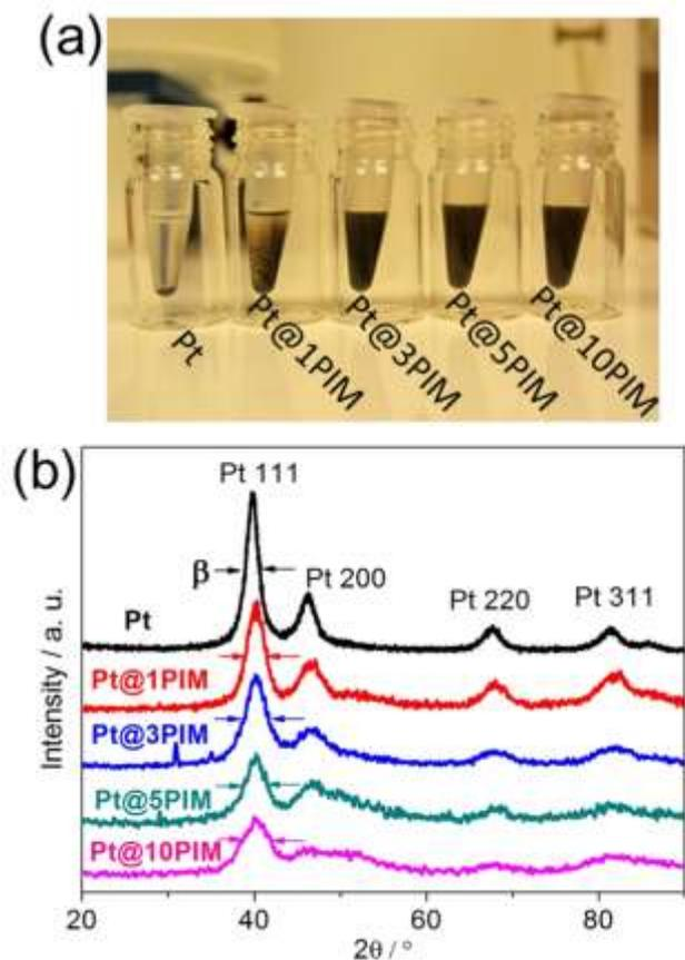
**Figure 2.** (a) Photographic image of Pt and Pt@PIM composites dispersed in ethanol after 12 h settling time. (b) XRD patterns of Pt and Pt@PIM composites. The 111 peak was used for estimating particle size from the peak width at half height  $\beta$ .
