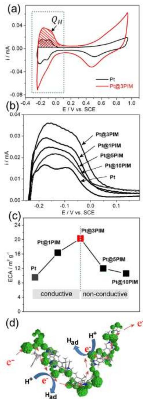
**Figure 5.** (a) Cyclic voltammograms (scan rate 0.05 Vs<sup>-1</sup>) for Pt and Pt@3PIM immersed in 0.1 M HClO<sub>4</sub>. (b) Hydrogen adsorption region within cyclic voltammograms for different samples. (c) Electrochemically active surface area (ECA) versus Pt@PIM sample. (d) Schematic mechanism of hydrogen adsorption/desorption in PIM-EA-TB stabilized Pt coupled to electrical conductivity.
