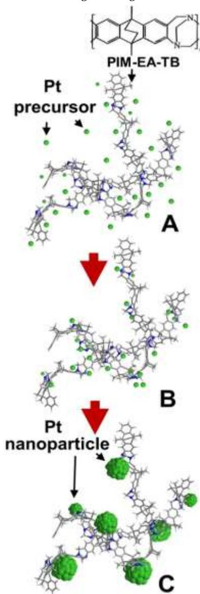
**Figure 1.** Schematic drawing of (A) Pt precursor diffusion into micropores, (B) adsorption to N-sites, and (C) the nucleation and growth of platinum nanoparticles in the presence of the rigid PIM-EA-TB capture agent (see molecular structure).
