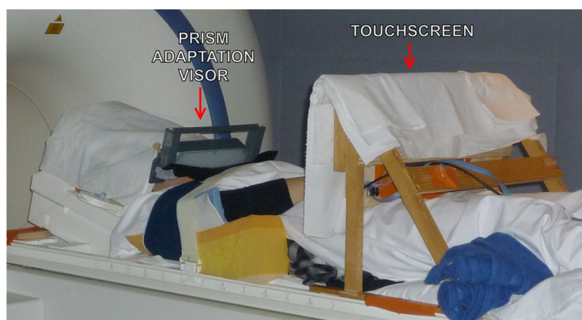
Fig. 1 Configuration for performing prism adaptation within the fMRI environment. Paper toweling around the head coil and black fabric along the bottom of the prism adaptation visor restricts the participant's field of view to that which can be seen through the window of the visor. The right arm is stabilized by cushions placed under and around the arm, and by straps securing the upper arm to the torso. Paper toweling is placed around the frame of the touchscreen to prevent it from providing a
