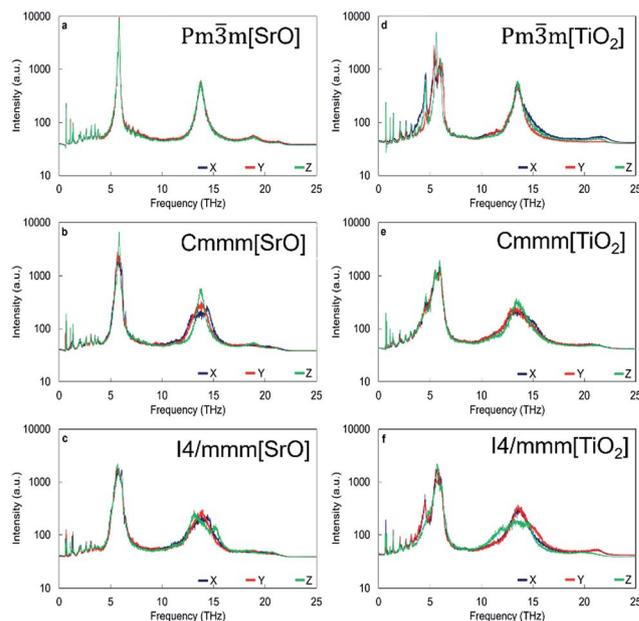
Fig. 6 HFACF spectra at 500 K of SrO-rich (a) *Pm3m*, (b) *Cmmm* and (c) *I4/mmm* assemblages and TiO<sub>2</sub>-rich (d) *Pm3m*, (e) *Cmmm* and (f) *I4/mmm* assemblages. The X, Y, Z components of the HFACF spectrum are shown in blue, red and green respectively. Intensity in arbitrary units on logarithmic scale. The temperature dependence of HFACF spectra displays the same features as for bulk SrTiO<sub>3</sub>.
