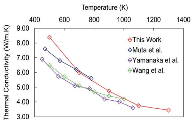
Fig. 3 Thermal conductivity of bulk SrTiO<sub>3</sub> calculated using the Green–Kubo method compared to experimental data.<sup>50–52</sup>
