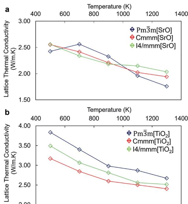
Fig. 4 Thermal conductivity of the (a) SrO-rich and (b) TiO<sub>2</sub>-rich nanocube systems, comparing the perfect stacking (*Pm3m*) with the displaced *Cmmm* and *I4/mmm* assemblages. Analysis of the three directional components of the thermal conductivity (*i.e.* *X*, *Y* and *Z*) does not show any relevant difference and therefore is not shown.
