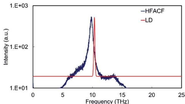
Fig. 8 HFACF spectrum at 500 K in log<sub>10</sub> scale and phonon DOS calculated neglecting the effect of temperature of stoichiometric SrO. Intensity in arbitrary units.
