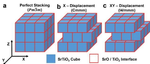
Fig. 1 Representation of self-assembly of SrTiO<sub>3</sub> nanocubes in (a) a perfect cubic stacking (*Pm* $\bar{3}$ *m*), and displaced assemblages of (b) an *X*-displacement configuration in the *X* direction of half a cube width relative to the neighbouring cube (*Cmmm*) and (c) an *XY*-displacement configuration in the *XY* plane of a quarter of a cube width relative to the neighbouring cube (*I4/mmm*). *X*, *Y* and *Z* are the directions of the unit cell.
