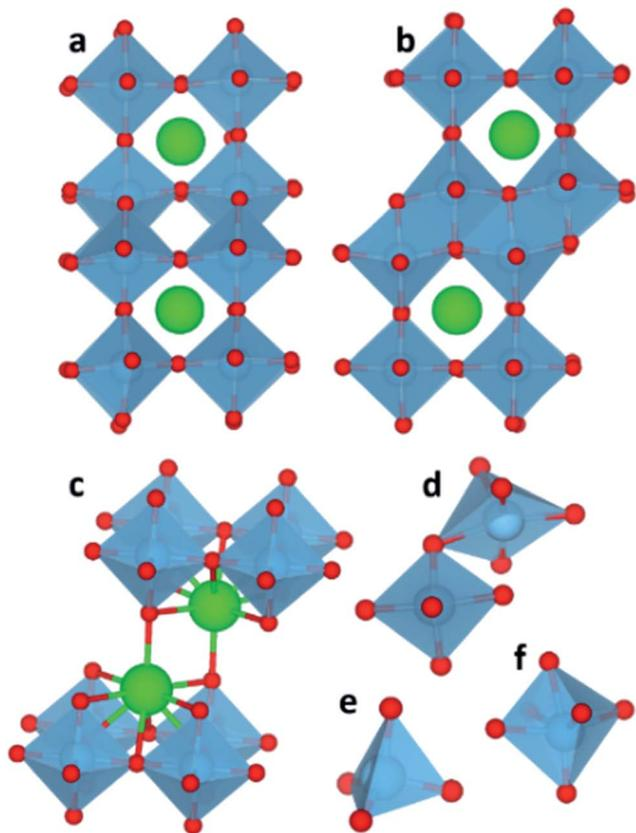
Fig. 2 The 12-fold coordination environment of Sr species at (a and b)  $TiO_2$ -rich interface and 9-fold at (c) SrO-rich interface. Coordination environments of Ti species at SrO and  $TiO_2$ -rich interfaces (d) dynamic octahedral coordination, (e) tetrahedral and (f) distorted octahedral.
