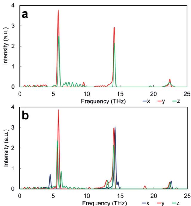
Fig. 7 Phonon DOS calculated neglecting the effect of temperature of thin film structures of (a) SrO-rich (Ruddlesden–Popper) and (b) TiO<sub>2</sub>-rich (Magneli) interface. Intensity in arbitrary units.
