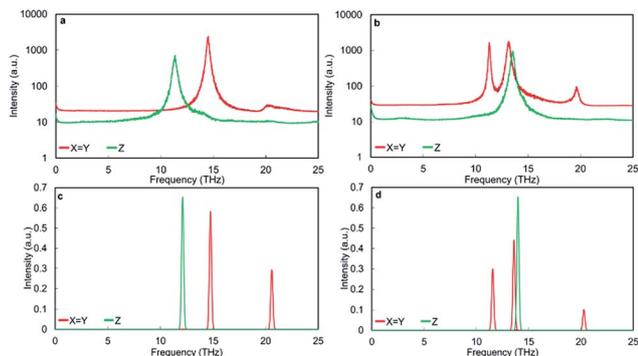
Fig. 9 HFACF spectra at 500 K of stoichiometric TiO<sub>2</sub> (a) anatase and (b) rutile. Phonon DOS calculated neglecting the effect of temperature of stoichiometric TiO<sub>2</sub> (c) anatase and (d) rutile. Intensity in arbitrary units for HFACF in log<sub>10</sub> scale. X, Y and Z are the directions of the unit cell and align with the crystallographic a, b, and c directions.
