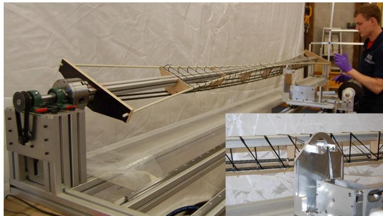
Figure 1: Filament winding of a W-FRP reinforcing cage.
