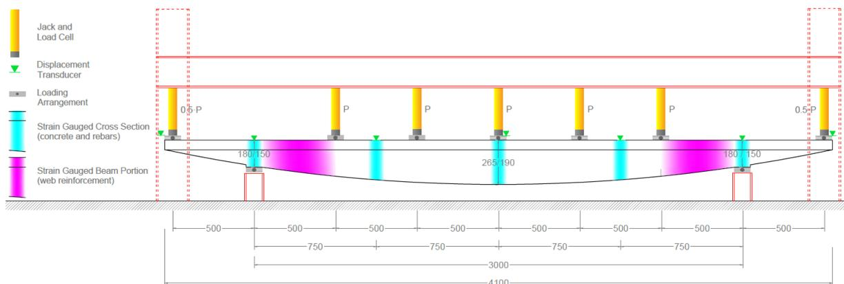
Figure 4: Experimental Setup.
