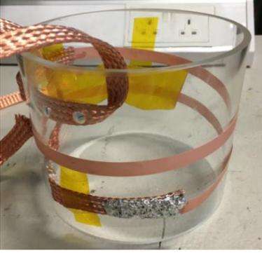
Fig. 1: YBCO tape wound onto a perspex tube.
