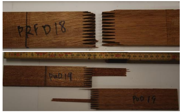
Figure 19: Failure of finger joints and wood for DRM specimens bonded with PRF (top) and PUR (bottom)
