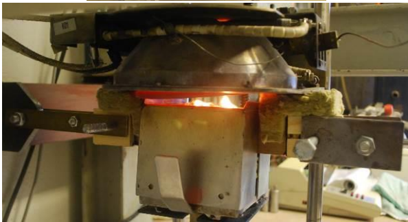
Figure 8: Bench-scale fire test with dead weights (top) and ignition (bottom)
