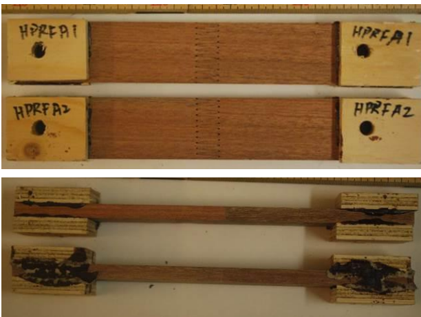
Figure 5: Reinforcement at the end sections
