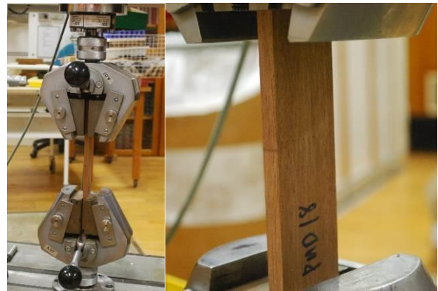
Figure 10: Tensile test in ambient temperature setup
