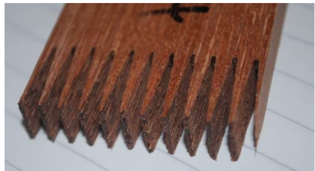
Figure 20: Mixture of wood fibre pull-out and adhesive failures in the glue lines
