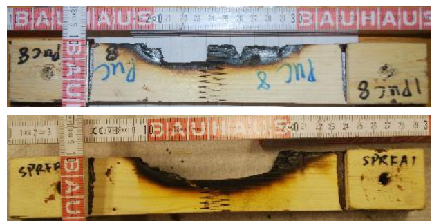
Figure 12: Typical failures of spruce finger joints bonded with PUR (top) and PRF (bottom) after fire tests
