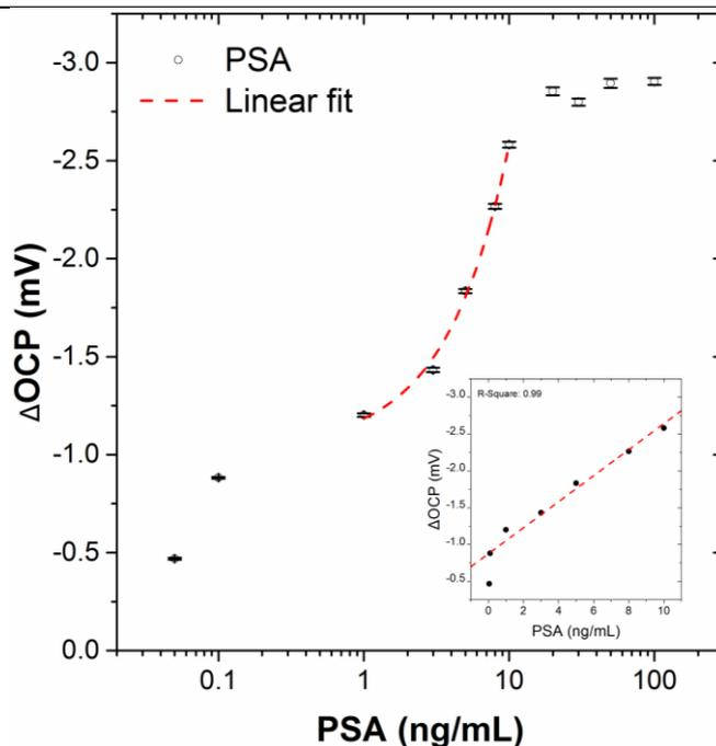
**Fig. 5** Dose response of the aptasensor. The points represent the average for 4 channels. The line represents a linear fit to the points between 1 and 10 ng/ml (as shown in the inset using a linear scale).
