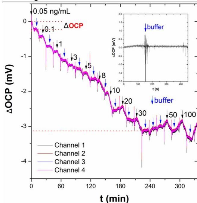
**Fig. 4** A typical OCP behaviour of the aptasensor with the response of consecutive injections of different concentrations of PSA (black arrows) and rinsing buffer (blue arrows) on four separate electrodes of the array. The numbers next to the black arrows indicate the PSA concentrations injected. The inset shows the initialization of the OCP measurement with an injection of buffer (blank solution).
