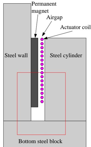
Fig. 2. Simplified model of the magnetic circuit
