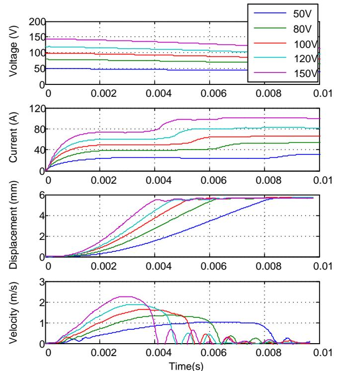
Fig. 14. Actuator opening operation with different capacitor voltages.
