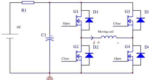
Fig. 11. Schematic diagram of the actuator control circuit.
