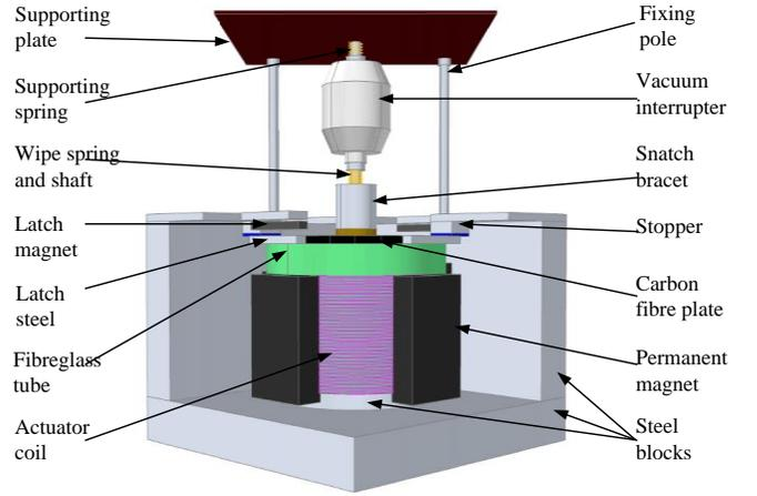
Fig. 9. 3-D structure of the operating actuator
