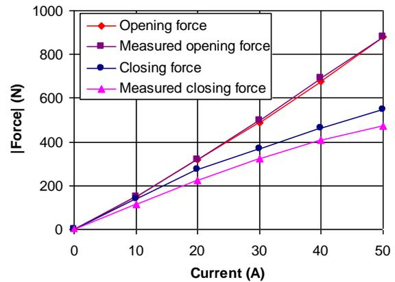
Fig. 13. Actuator opening and closing force versus current.
