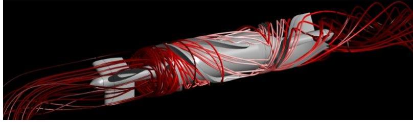
**Figure 5:** Pathlines through the HeartMate II VAD
