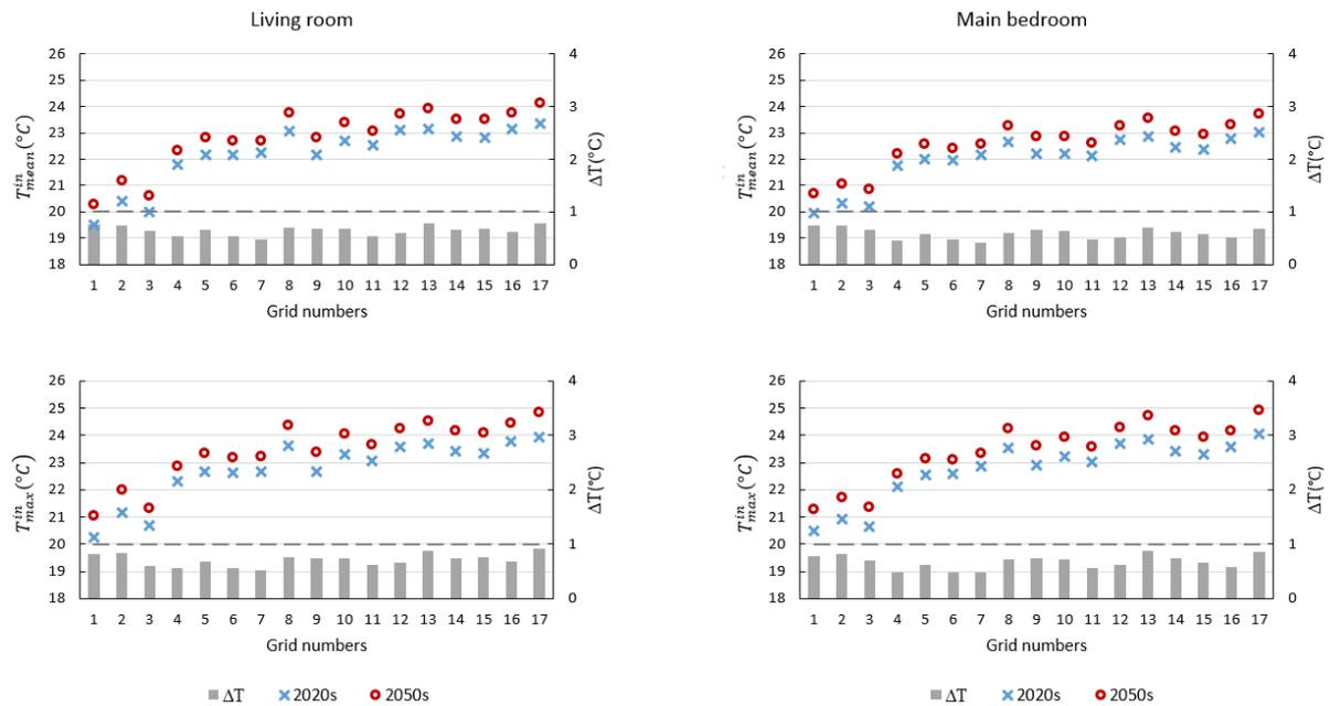
Figure 5. Variation in the median  $T_{mean}^{in}$  and  $T_{max}^{in}$  across the city in the 2020s and in 2050s.  $\Delta T$  shows the increase in  $T_{mean}^{in}$  (or  $T_{max}^{in}$ ) by the 2050s compared to the 2020s.
