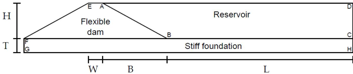
Figure 3: Geometry of the trapezoidal earth dam considered.
