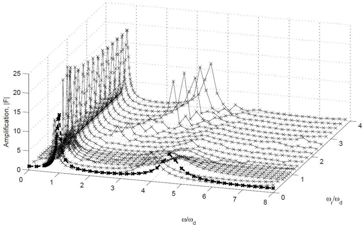
Figure 4: Amplification of acceleration,  $|F|$  at the crest of the rectangular concrete dam for various values of the frequency ratios  $\omega/\omega_d$  and  $\omega_r/\omega_d$  (After Pelecanos et al. [32]).
