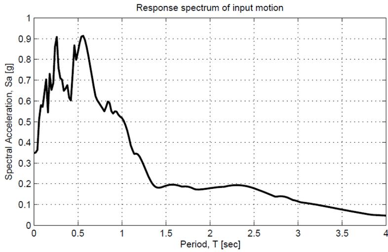
Figure 7: Response spectrum of the El Centro (1940) earthquake record for damping  $\xi=5\%$ .
