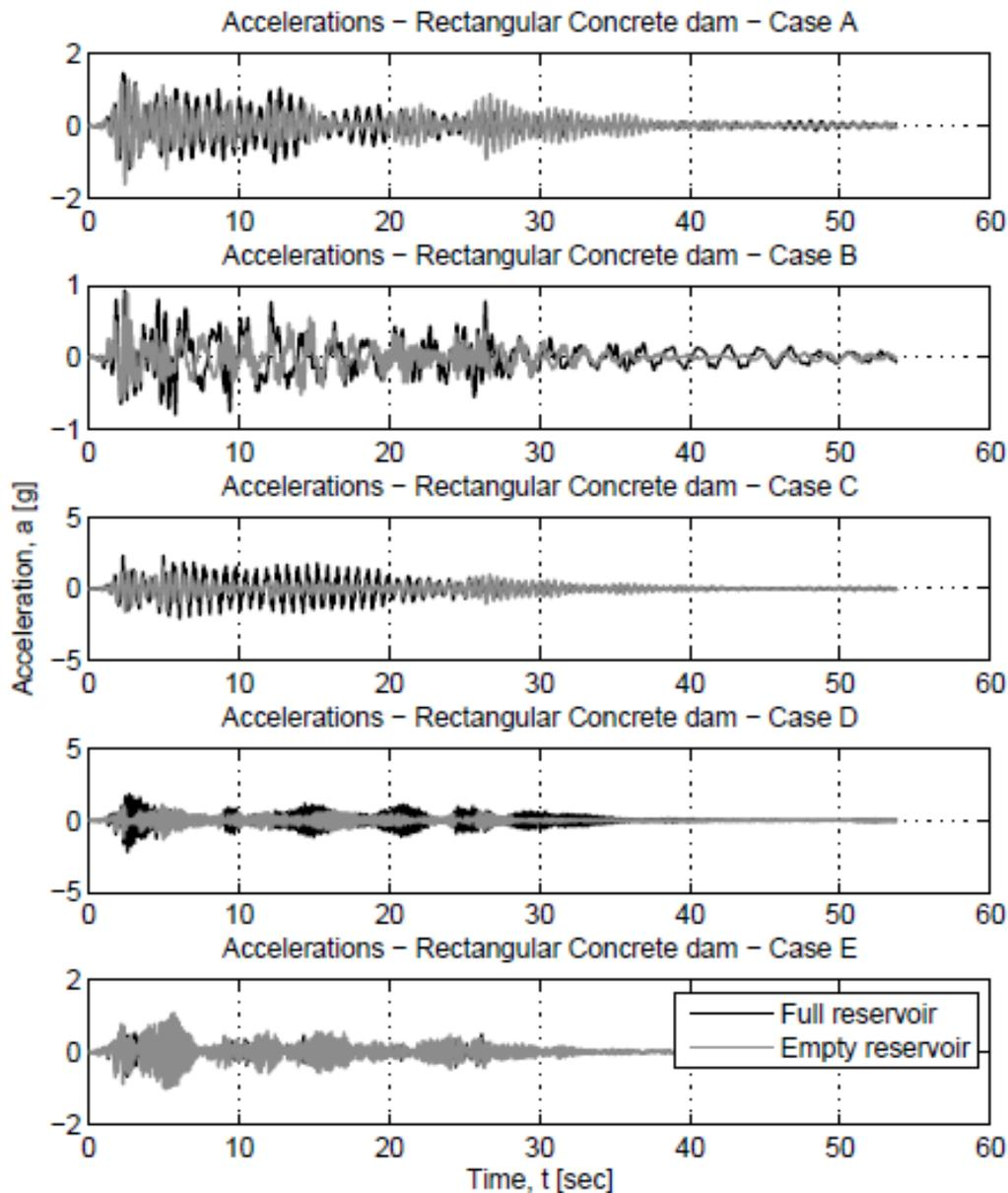
Figure 9: Acceleration time-histories at the crest of the rectangular concrete dam.
