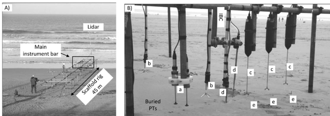
**Figure 3. Images showing the scaffold frame (A) and the main instrument bar (B). Sensors on the main instrument are: electromagnetic current meters (a), Vectrino I velocimeters (b), Vectrino II acoustic Doppler current profilers (c), FOBS (d) and CCPs (e). The buried Pressure transducers (PTs) and in situ bed cam are only identified by their names in the photo.**
