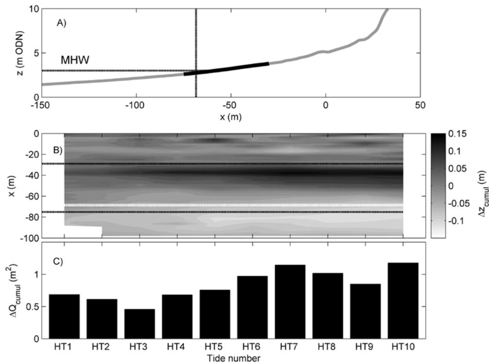
**Figure 5. Morphologic variability during the BeST study. A) Beach profile from October 13, 2011 with scaffold frame identified in black. B) Cumulative elevation change for each tide. Horizontal black lines indicate seaward and landward edges of the scaffold frame. Horizontal white line indicates the location of the main instrument bar. C) Cumulative volumetric flux integrated over the tidal cycle and cross-shore distance.**
