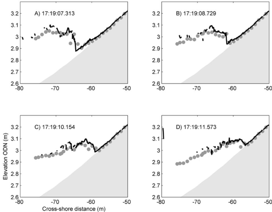
**Figure 6. Comparison between UDM (dots) and LiDAR (black curves) for several instances of uprush motion identified by hours:minutes:seconds.milliseconds. Shaded area identifies the beach as determined from the post-tide 7 profile.**
