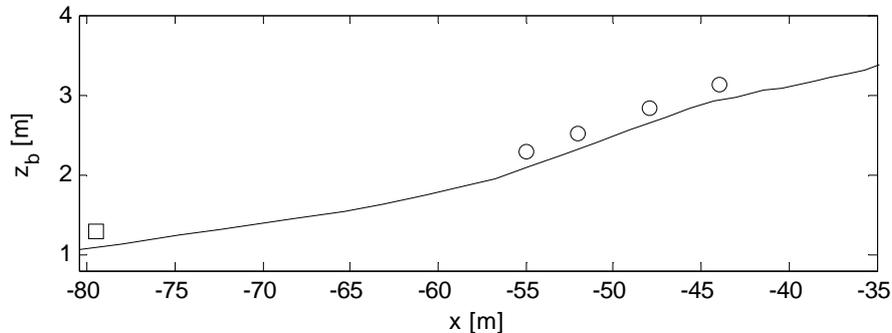
**Figure 1. Measurement locations along the coastal bottom profile (and model domain) used for comparison with model output (where the vertical axis represents bed level height and the horizontal axis is the cross-shore distance). The square represents the (offshore) PT/ADV, while the circles represent the acoustic bed level sensors in the swash.**
