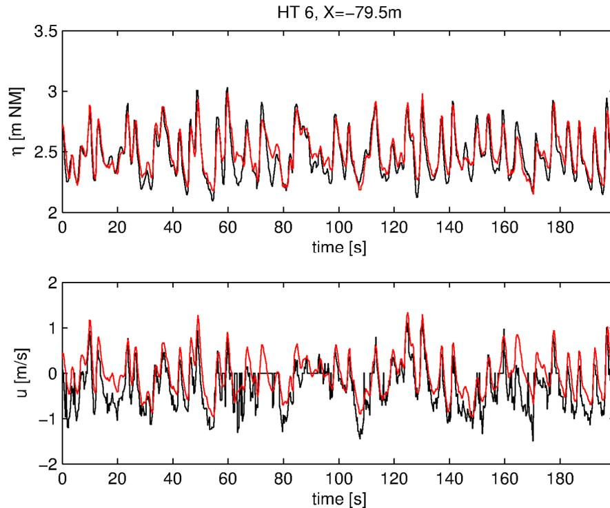
Figure 3. Top panel: comparison between measured (black) and computed (red) water surface elevation (in meter with respect to MSL) at the offshore model boundary ( $x = -79.5\text{m}$ ) for a 200s time window during HT 6. Bottom panel: idem for the velocity.
