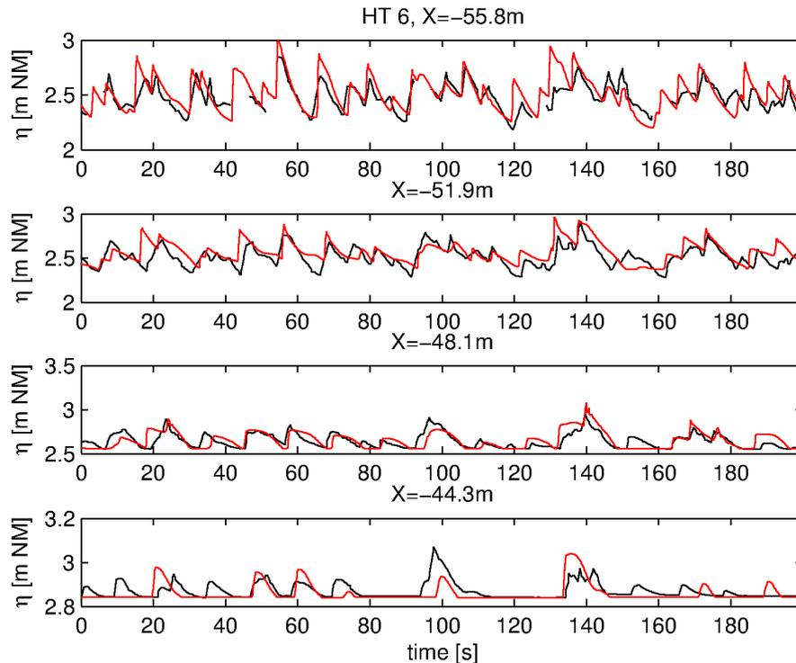
Figure 5. Comparison between measured (black) and computed (red) water surface elevation time series at the four locations in the swash zone during HT 6.
