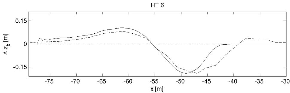
**Figure 7. Measured (dashed line) and computed (solid line) total bed level changes along the cross-shore profile during tide 6, where positive (negative) bed level changes indicate accretion (erosion).**
