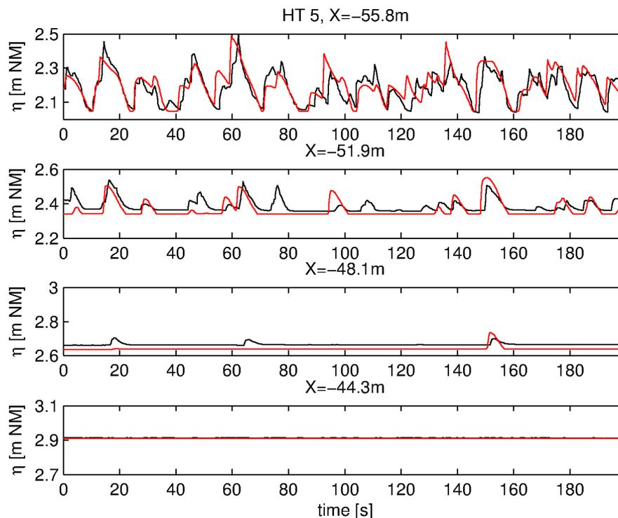
Figure 4. Comparison between measured (black) and computed (red) water surface elevation time series at the four locations in the swash zone during HT 5.
