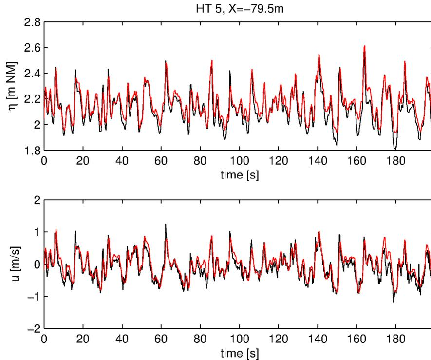
Figure 2. Top panel: comparison between measured (black) and computed (red) water surface elevation (in meter with respect to MSL) at the offshore model boundary ( $x = -79.5\text{m}$ ) for a 200s time window during HT 5. Bottom panel: idem for the velocity.
