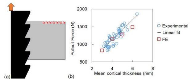
Figure 2: Experimentally measured pullout forces and FE predictions for varying cortical thickness using screws inserted with 1Nm torque.
