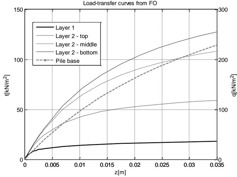
Figure 3. Back-calculated load-transfer curves for the soil springs.
