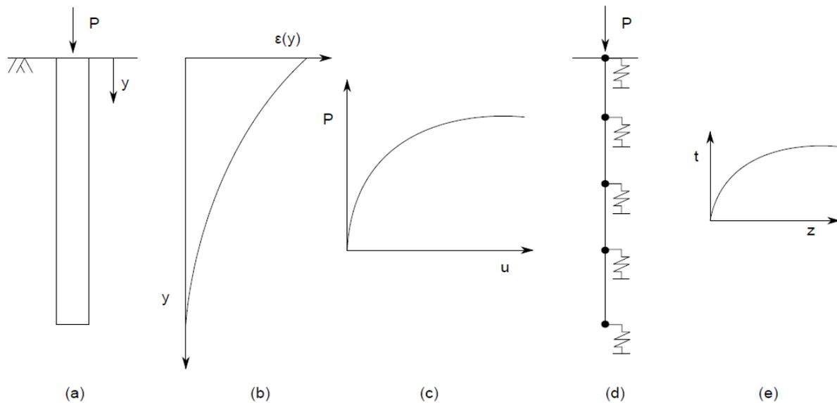
**Figure 1.** Problem definition: (a) axially loaded pile, (b) profiles of axial strain for each load step, (c) pile top load-displacement curve, (d) finite element beam-spring model of the pile-soil interaction and (e) load-transfer curve defining the nonlinear behaviour of a soil spring.
