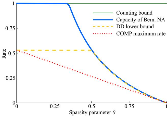
Fig. 1. Graph showing group testing rates with  $k = \Theta(n^\theta)$  defectives: the trivial counting bound  $C \leq 1$ ; the capacity of Bernoulli nonadaptive group testing (Theorem 2); an achievable rate of the DD algorithm (10) [1]; and the maximum achievable rate of the COMP algorithm with Bernoulli tests (Corollary 2)
