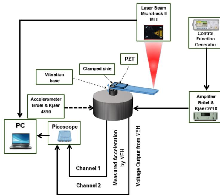
Figure 1. A configuration of the test station for vibration-based energy harvester.
