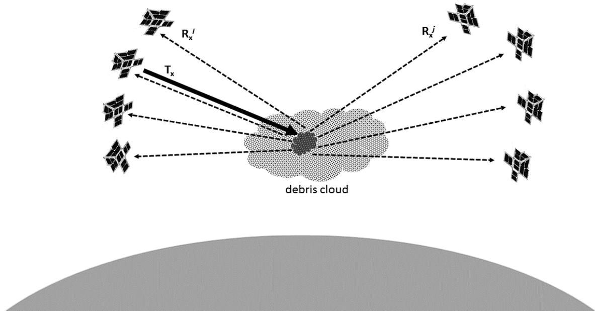
Figure 3. One of the many constellation geometries used to detect/image debris clouds. One satellite ( $T_x$ ) is transmitting an EM wave, received by all other satellites ( $R_x$ ) to provide a multistatic description of relevant parts of the debris cloud. Satellites can switch between receive/transmit modes and some will have additional processing capabilities. Generic CubeSat design adapted from <http://aprs.org/psat/cube-hinge2.GIF>.
