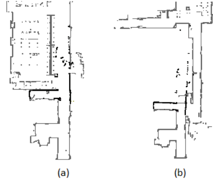
Fig. 3. Calculating localisation score by comparing laser rangefinder data (black) to (a) the correct floor map (grey), (b) an incorrect floor map
