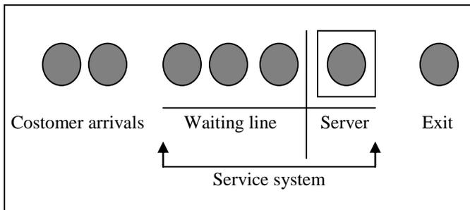
Figure 1. A generic representation of a service process.
