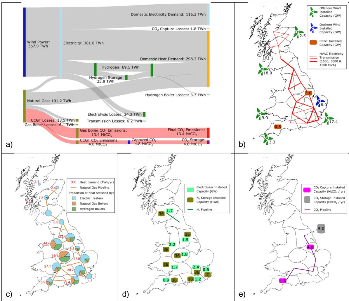
Figure 1: An optimal network design for Great Britain in 2050: (a) Sankey diagram of energy and CO<sub>2</sub> flows; (b) new and existing network for electricity supply; (c) new and existing network for provision of heat; (d) new hydrogen network; and (e) new CCS facilities.
