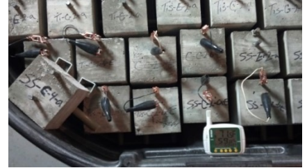
c) electrically coupled specimens and T/RH sensor
