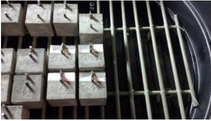
a) support of specimens in GFRP rack
