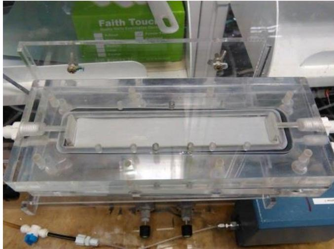
Figure 3.2: Photograph of the filtration cell used in the critical flux chapter of this work
