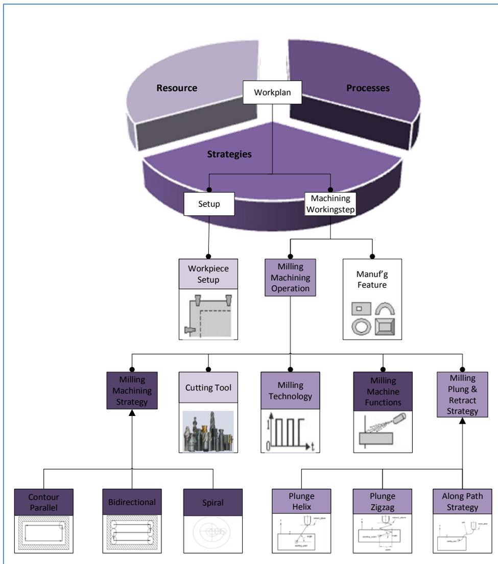
Figure 6.6 - STEP-NC representation of manufacturing information
