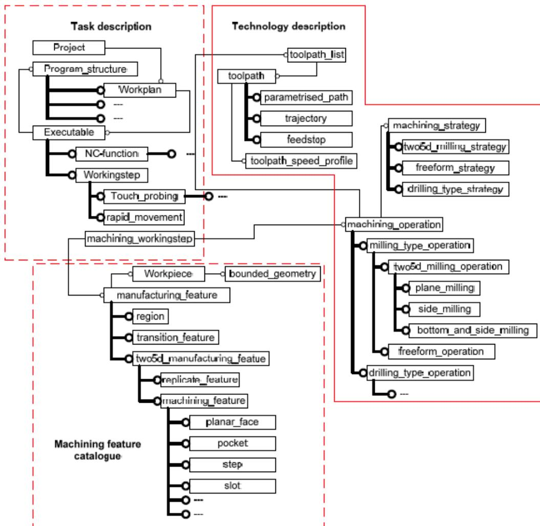
Figure 6.4 - Data structure of ISO14649 (STEP-NC) standard (Suh and Cheon, 2002)
