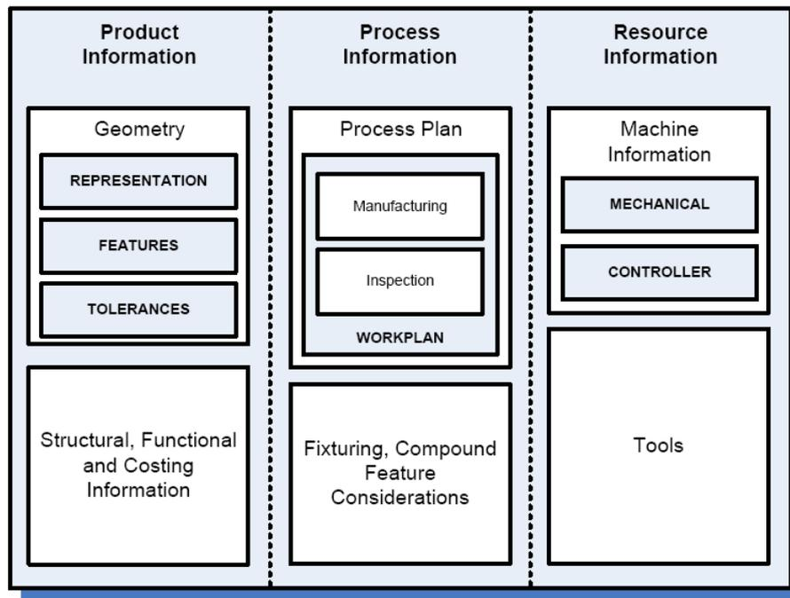
Figure 6.2 - Information category for a milled component in CNC manufacture (Nassehi, 2007)
