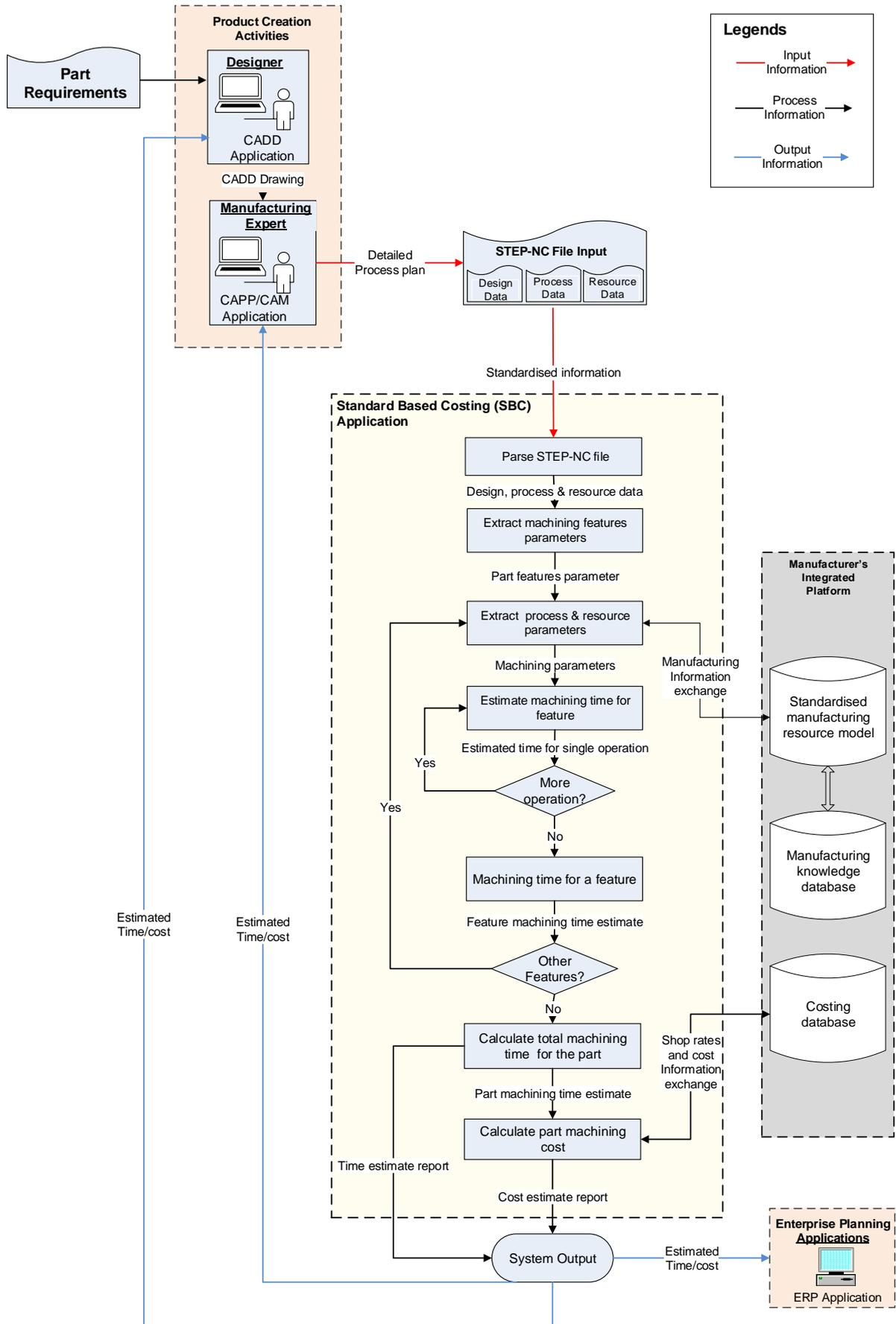
Figure 7.5 - Process flow for the SBC prototype
