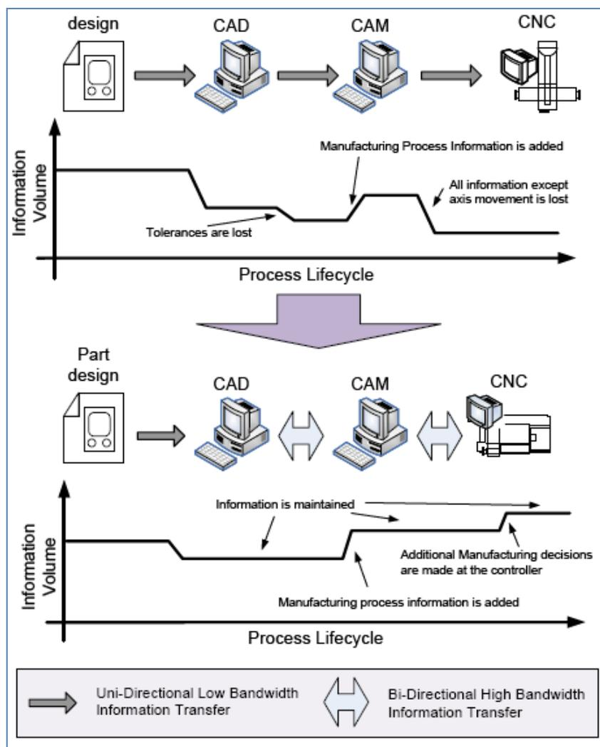
Figure 6.7 – Increasing information in STEP-NC compliant CNC manufacture (Nassehi 2007)
