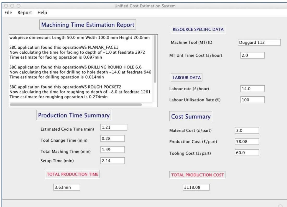
Figure 9.3 – SBC system time and cost estimation result display for part 1
