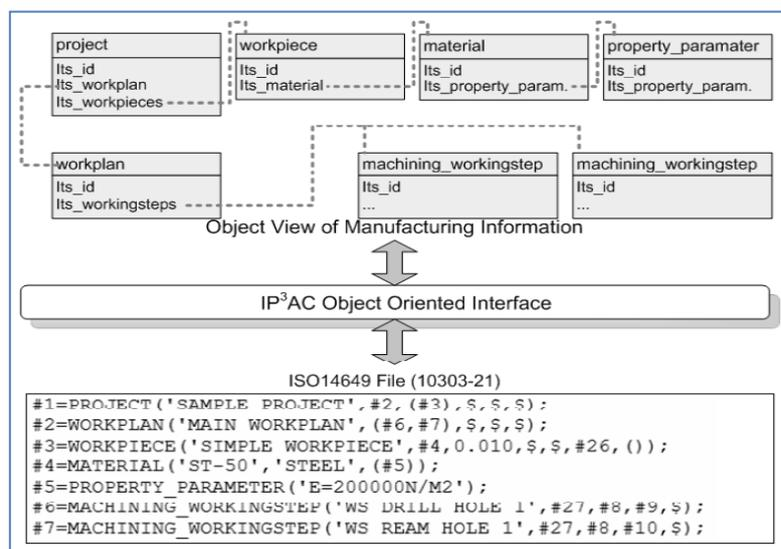
Figure 6.11 - Objects encapsulation of product creation information in IP<sub>3</sub>AC (Nassehi, 2007)
