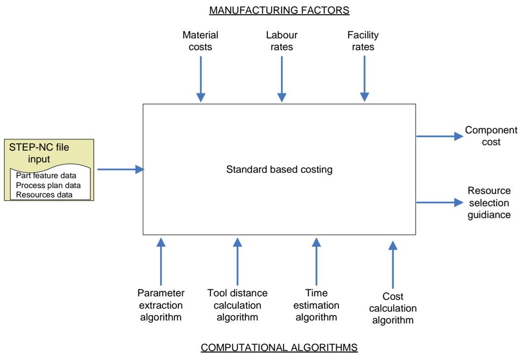
Figure 6.9 - IDEF0 diagram of STEP-NC compliant costing framework
