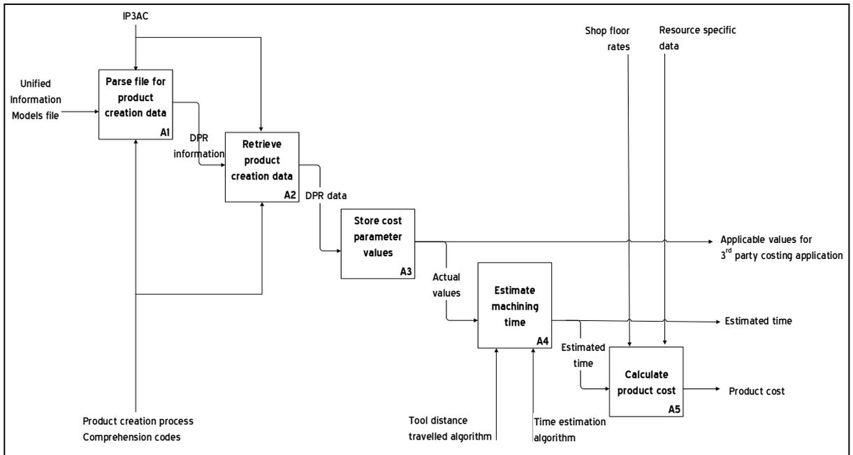
Figure 6.12 – Functional overview of an information model based Unified costing framework
