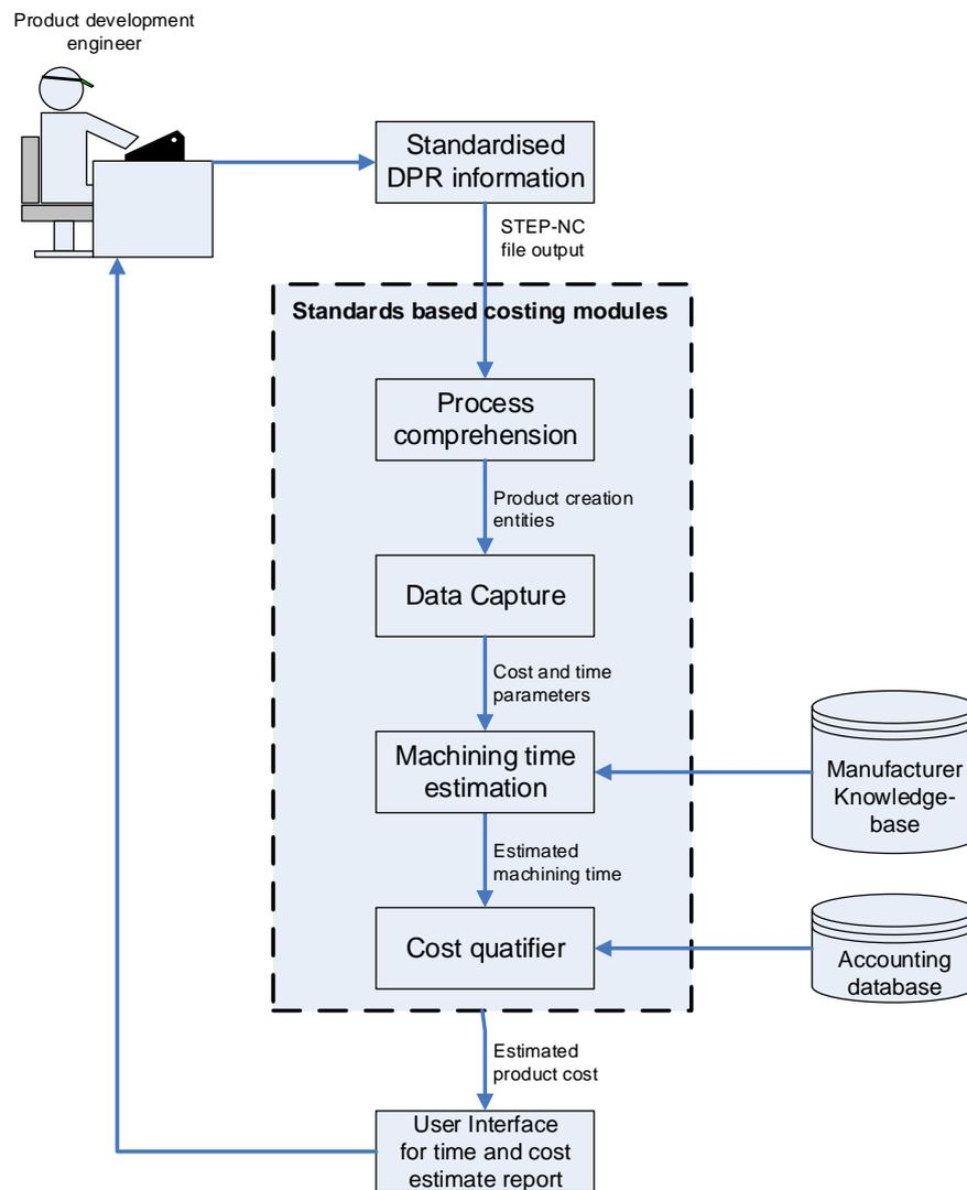
Figure 7.4 - Conceptual model of unified cost estimation
