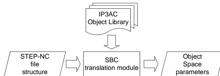
Figure 7.6 - Information translation by standard compliant costing framework
