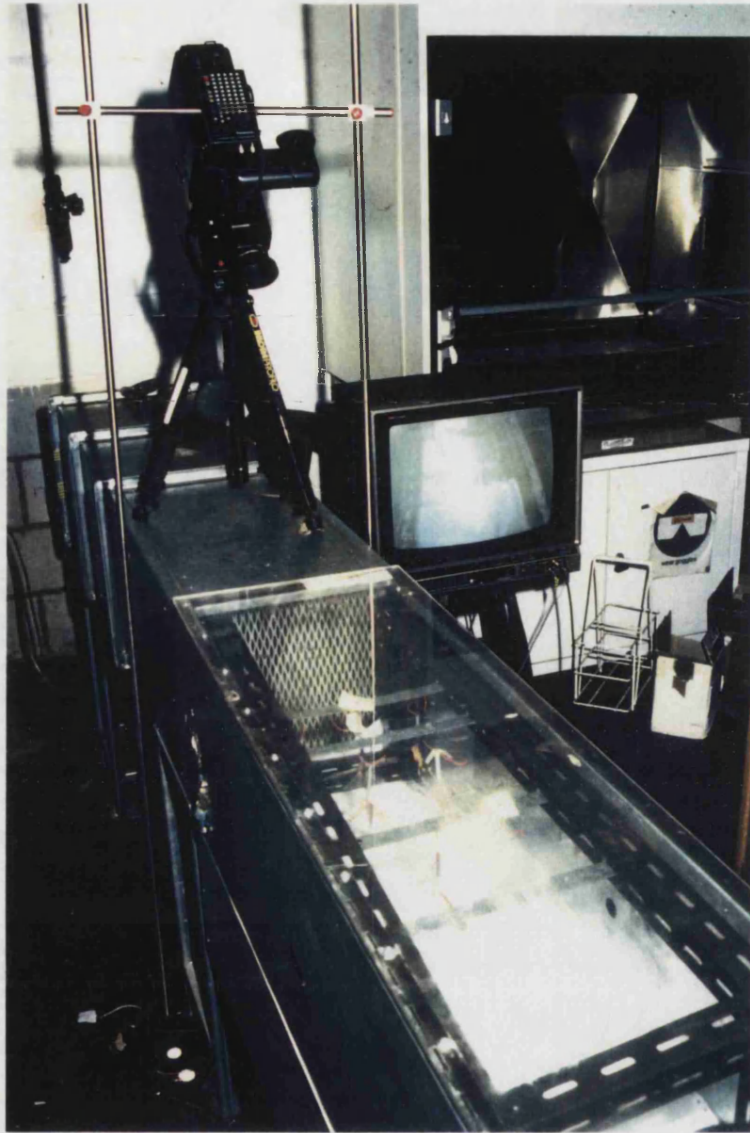
Plate 6.1. Flying locusts in wind tunnel. Flight being recorded with a camcorder. Note image on TV monitor.
