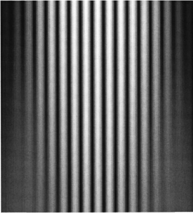
FIG. 3. Fundamental amplitude due to cosine grating (intersecting beams) in plane  $y=0$ . Beam propagates down the page from grating at the top. FSD=1 MPa. Region shown is 67 by 150 mm<sup>2</sup>, expanded  $\times 2$  horizontally.
