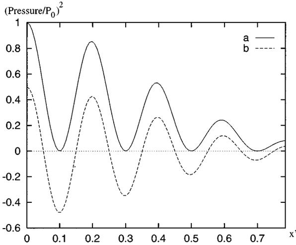
FIG. 8. Illustrating a mechanism for the production of fingers; (a) the square of the source function  $W_1(x',0)$ , for  $K=10\pi$ , to which the second harmonic is initially proportional and (b) the same function with an offset of half the envelope  $\exp(4x'^2)$ . (b) Possesses fingers at  $x'=0.1, 0.3, \dots$ .
