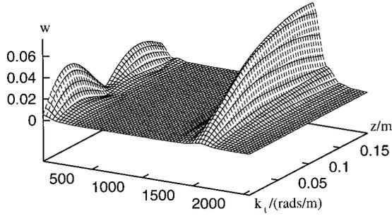
FIG. 5. Amplitude of the transverse Fourier transform of the second harmonic, as a function of  $z$ , the distance from a cosine grating. The units of  $k_x$  are rad/m, the fundamental having a maximum at  $k_x = K/a = 785$  rad/m, which generates second harmonic components at  $\pm K/a \pm K/a$ .
