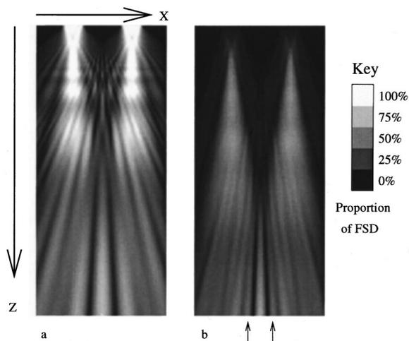
FIG. 1. Amplitude plot of Young's fringes, showing a region 33 mm wide, the beams propagating down the page for 150 mm. The images are expanded  $\times 2$  horizontally. (a) Fundamental, full scale deflection (FSD)=1 MPa, (b) second harmonic, FSD=0.5 MPa. Two fingers are indicated by arrows.
