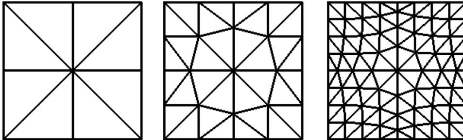
Figure 3: Simple square mesh showing constrained subdivision.
