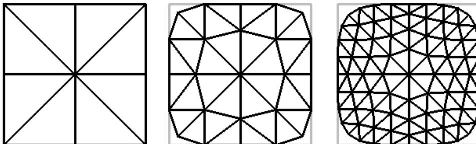
Figure 2: Simple square mesh showing unconstrained subdivision.
