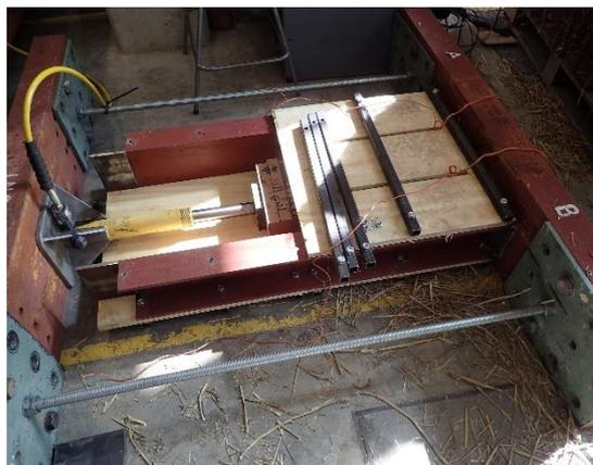
Fig. 3: Set-up for compacting prototype bales
