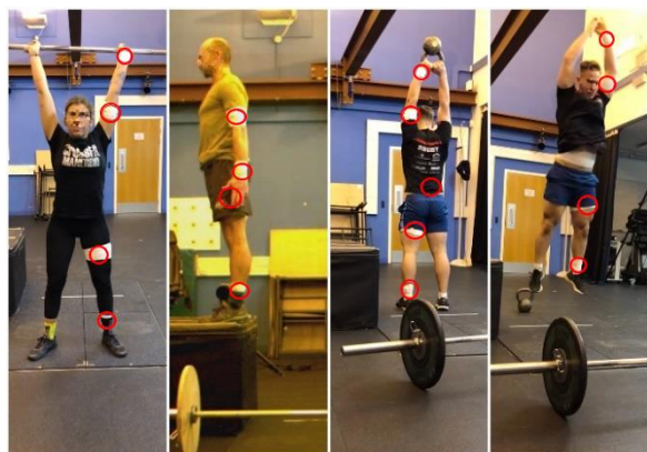
Figure 1: Setup used for the acquisition of the functional training drills. Red circles highlight sensors positions.
