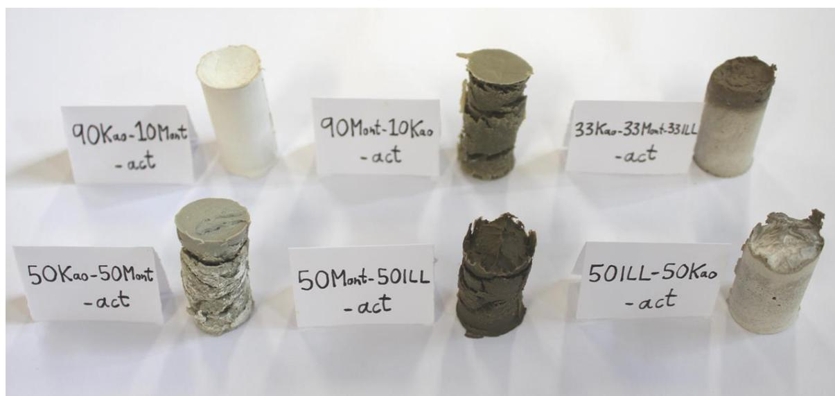
Figure 2: Photos of the cured activated mixed clay samples.
