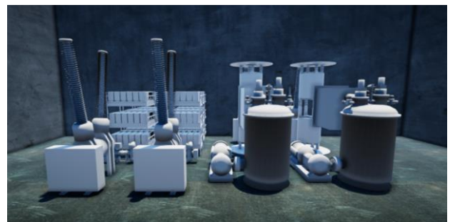
Figure 7: Visualisation of HVDC Breaker
