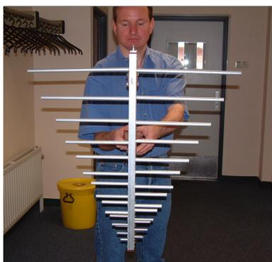
Fig. 2. The 200 MHz to 1 GHz Log-Periodic Dipole Antenna.
