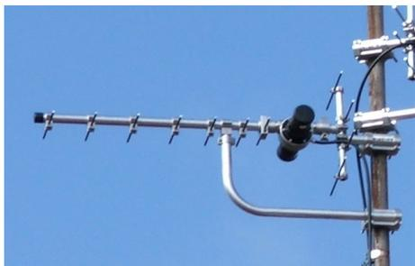
Fig. 1. The 12 elements UHF Yagi-Uda antenna.
