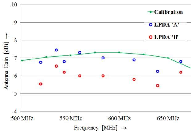
Fig. 7. Comparison of external calibration values of the LPDA's with the antenna gain obtained with Distance Scan.
