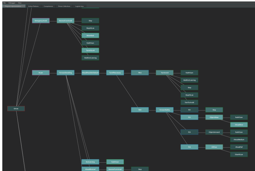
Fig. 1 The ABOD3 Graphical Transparency Tool displaying a POSH plan for a mobile robot, in debugging mode. The highlighted elements are the ones recently called by the planner. The intensity of the glow indicates the number of recent calls.
