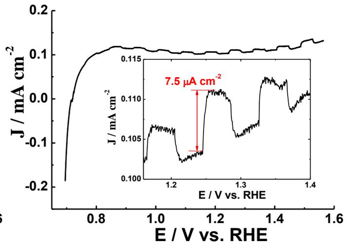
Fig.4. Cyclic voltammety (scan rate  $2.5 \text{ mV s}^{-1}$ ) for  $\text{SnO}_2\text{-Sb}_2\text{O}_5$  ceramics under chopped blue light (0.03 Hz) at the increase potential. The inset presents a part of the same cyclic voltammety in magnification.
