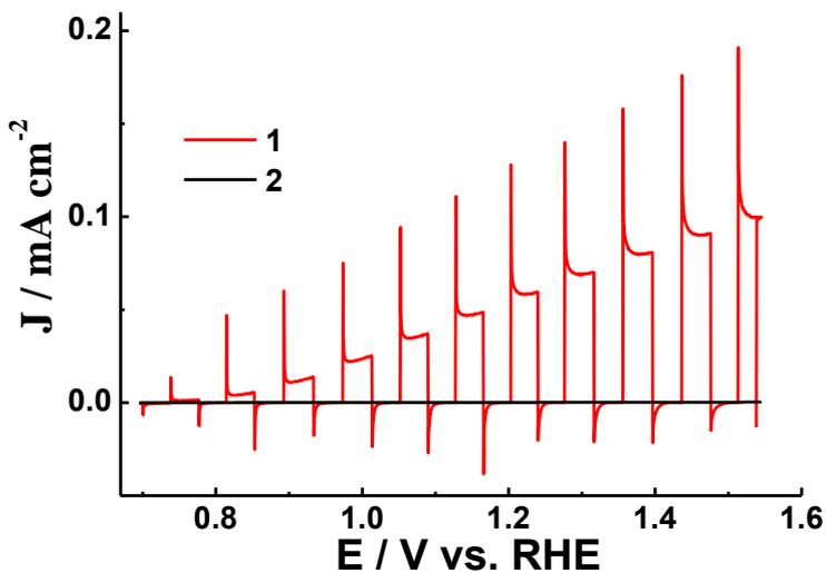
Fig.5. Cyclic voltammety (scan rate  $2.5 \text{ mV s}^{-1}$ ) for a hematite photoelectrode grown on ITO substrate at the increase potential (curve 1) and its decrease (curve 2). Curve 1 was recorded under chopped blue light (0.03 Hz), and curve 2 when light was off (the dark current).
