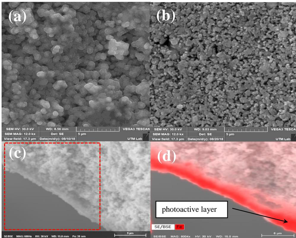
Fig.2. SEM micrographs of the photoelectrode: (a)hematite coating on  $\text{SnO}_2\text{-Sb}_2\text{O}_5$  ceramics; (b) $\text{SnO}_2\text{-Sb}_2\text{O}_5$  ceramics on reverse side of photoelectrode; (c) cross-sectional of photoelectrode; (d) EDS elemental map of the Fe distribution in ceramic substrate for the selected area (red square) in (c).
