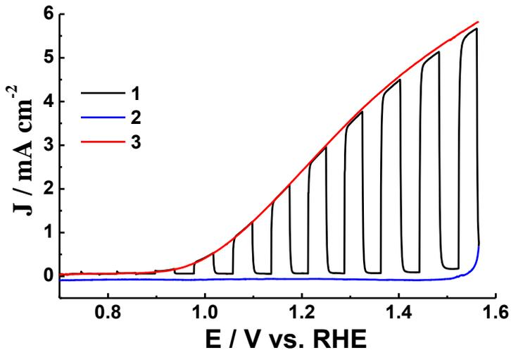
Fig.3. Cyclic voltammety (scan rate  $2.5 \text{ mV s}^{-1}$ ) for a hematite photoelectrode at the increase potential (curves 1 and 3) and its decrease (curve 2). Curve 1 was recorded under chopped blue light (0.03 Hz), curve 2 when the light was off (the dark current) and curve 3 when blue light was permanently on.
