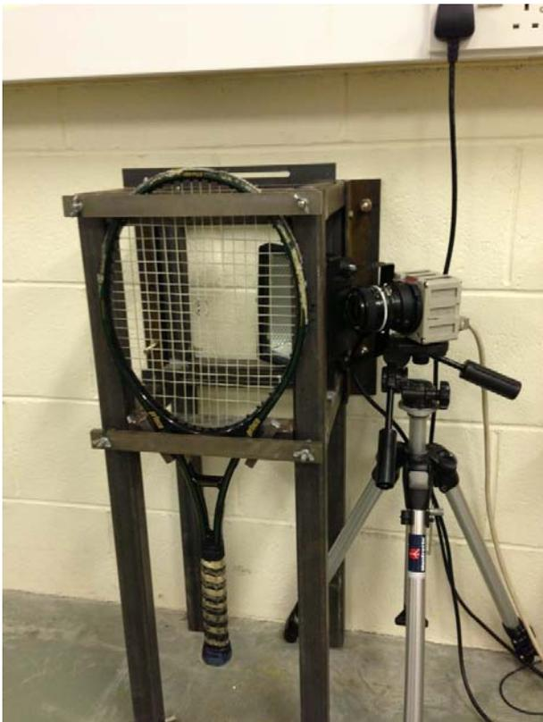
**Figure 5.** Experimental set-up showing a head-clamped racquet and HSC
