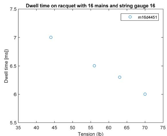
**Figure 13** Dwell time between a 'tournament' nylon string and a 'used' pressured ball
