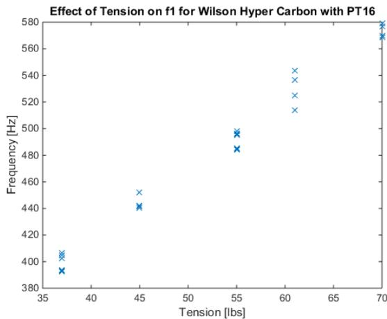
**Figure 8** Effect of string tension on frequency of a racquet with 16 mains strings strung with polyester.
