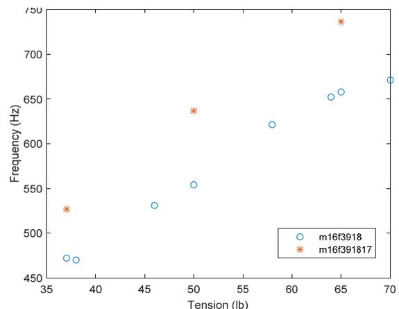
**Figure 11** Effect of string tension and string gauge on frequency
