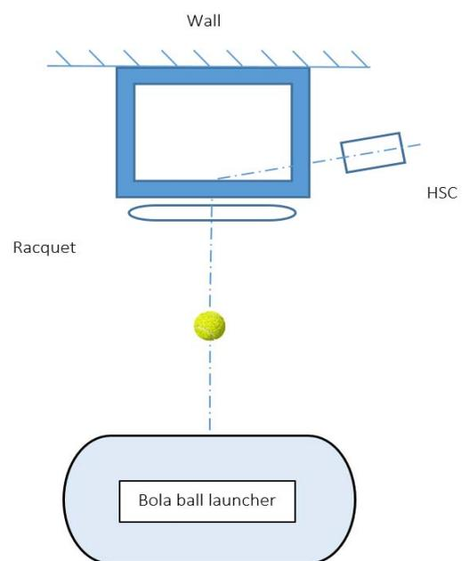
**Figure 3** Layout of the experiment showing the position of the high-speed camera to the racquet
