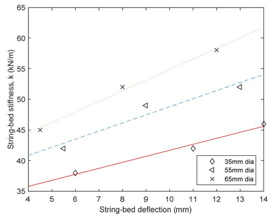
**Figure 1** Experimental data for string-bed stiffness, determined by applying a distributed force perpendicular to the string plane [9]
