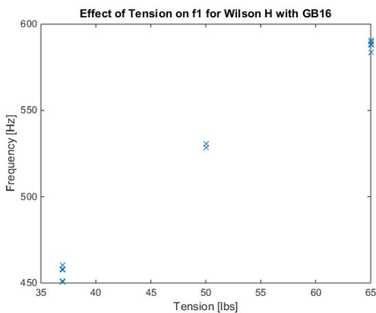
**Figure 9** Effect of string tension on frequency of a racquet with 16 mains strings strung with natural gut.
