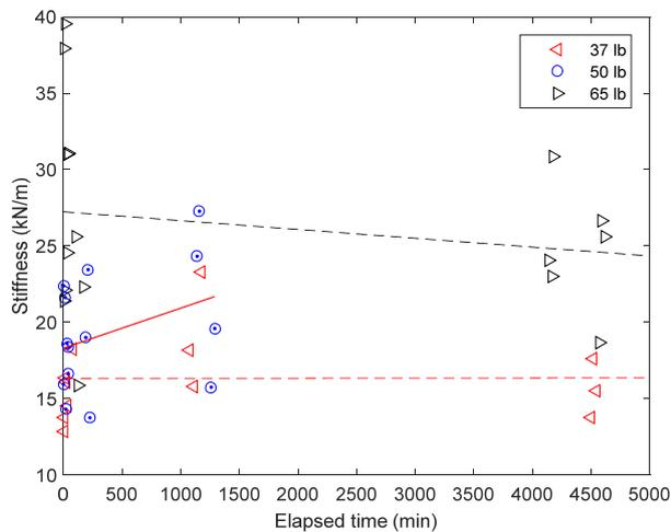
**Figure 14** Dynamic stiffness over time since being strung for a mid-size racquet at three different initial tensions.
