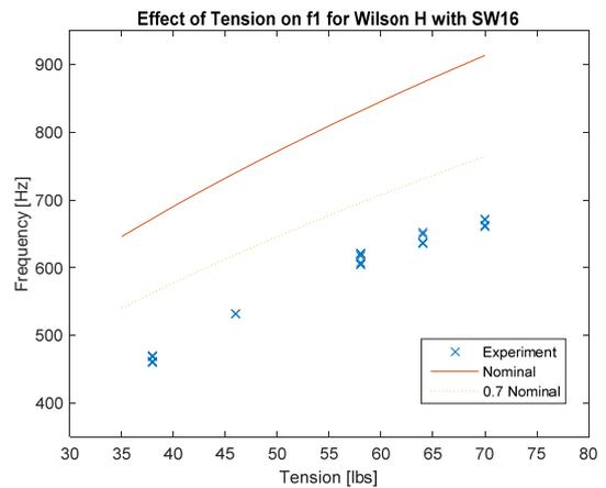
**Figure 10** Comparison of theoretical frequency with no tension loss and a 30% tension drop after stringing against experimental results for synthetic gut, 16 gauge
