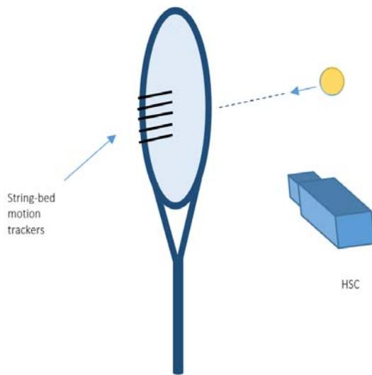
**Figure 2** Measurement of maximum string-bed displacement using aluminium trackers
