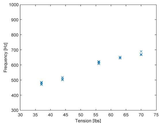
**Figure 7** Effect of string tension on frequency of a racquet with 16 mains strings strung with a 'tournament' nylon.
