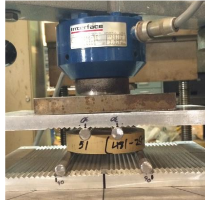
b) test being conducted in universal test machine (shown: 100 mm diameter culm tested over 80 mm span with 25 mm shear span)
