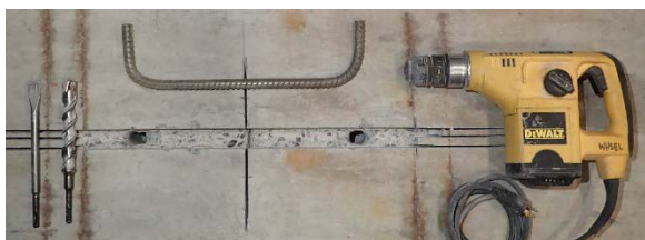
Staple, channel and installation tools
