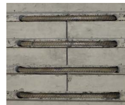
TiNSM4 staples before epoxy embedment
