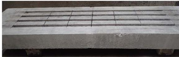
NSM channels on [inverted] slab soffit; transverse cuts through internal reinforcing bars can also be seen.
