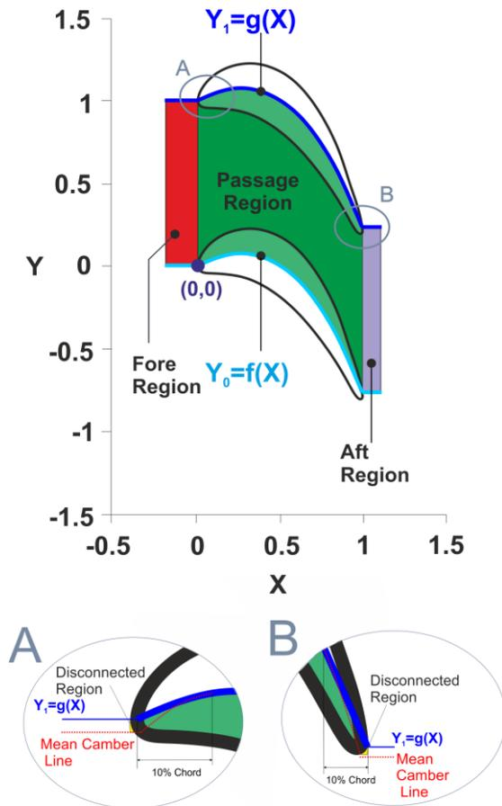
**Figure 2 A cascade view of a generic vane/blade profile at the hub with endwall regions identified.**
