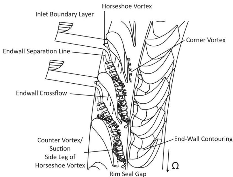
**Figure 1 Secondary flow features in a turbine annulus.**
