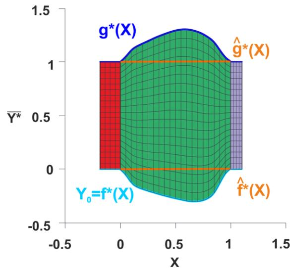
**Figure 12 Representation of the vane/blade profile in the orthonormal domain using a rescaled  $\bar{Y}^*$ .**
