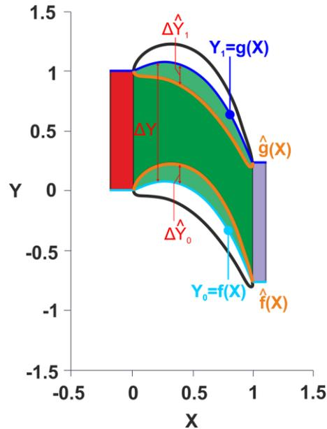
**Figure 8 A cascade view of a generic blade profile identifying the blade-endwall intersections (note: the mesh lines have been omitted here for clarity).**
