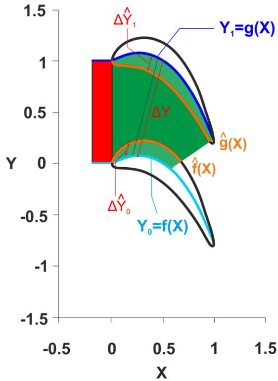
**Figure A1: A cascade view of a generic blade profile identifying the blade-endwall intersections for an inter-blade passage mesh that terminates at the throat (note: the mesh lines have been omitted here for clarity)**
