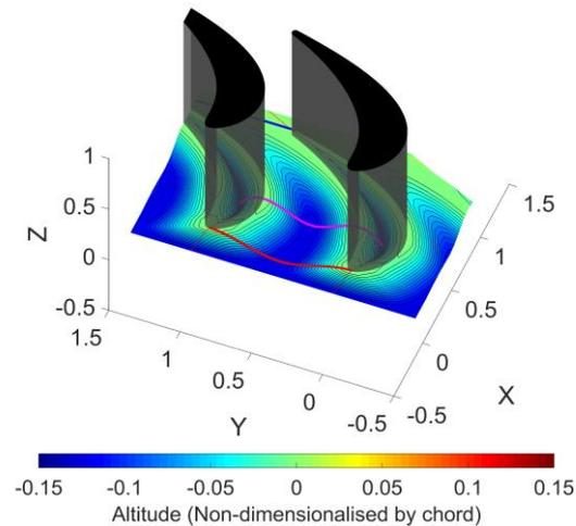
**Figure 15 Cascade representation of the generated endwall surface.**
