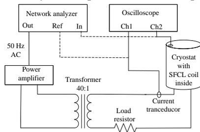
Fig. 4. AC loss measurement circuit schematic
