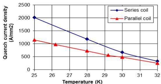
Fig. 10. Quench current density versus temperature (self-field)
