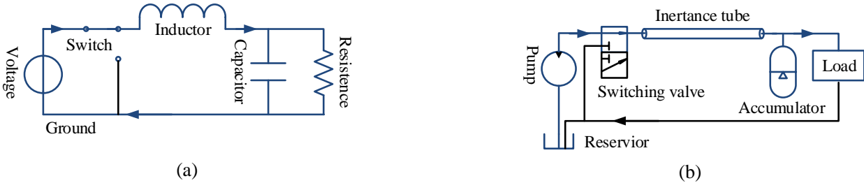
Fig. 1: Electrical buck converter and a three-port SIHC
