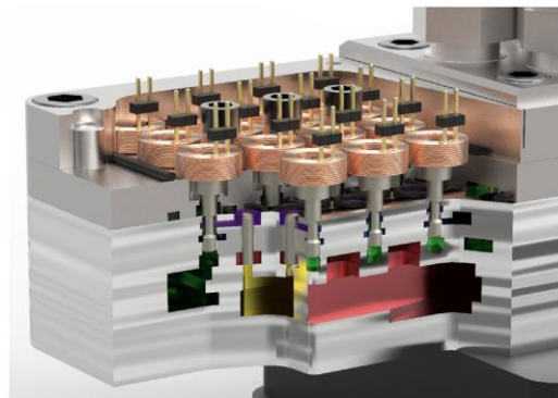
b) A miniature valve system in 2017 [63]
