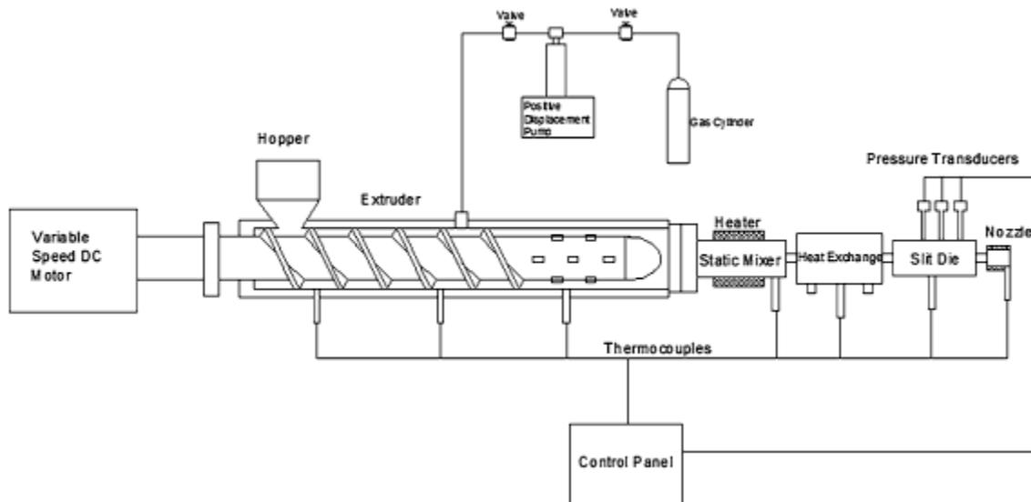
Figure 9. Schematic of the extruder set up for the measurement of WPC/supercritical CO<sub>2</sub> solution viscosities [50].
