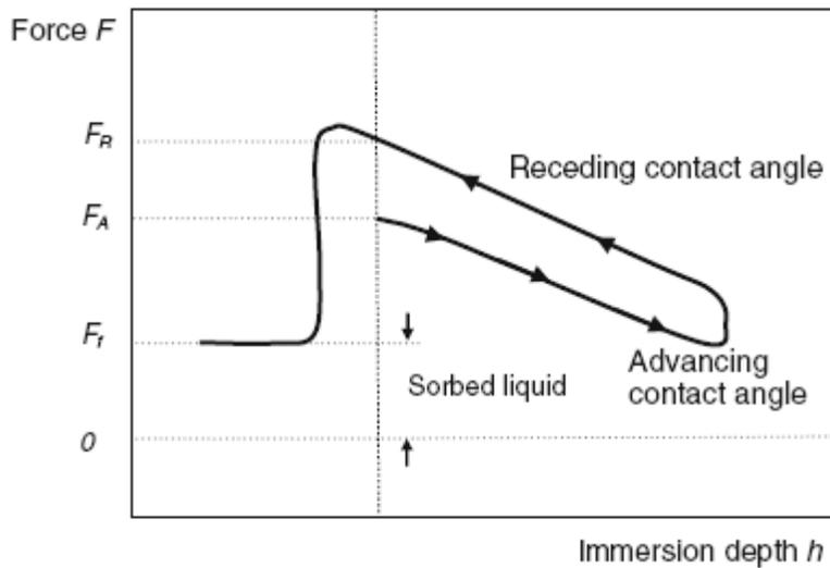
Figure 2. Schematic of force  $F$  versus immersion depth  $h$  for Wilhelmy plate test . Forces  $F_A$  and  $F_R$  are obtained from the advancing and receding curves respectively and the final force  $F_f$  corresponds to the mass of absorbed liquid [8].
