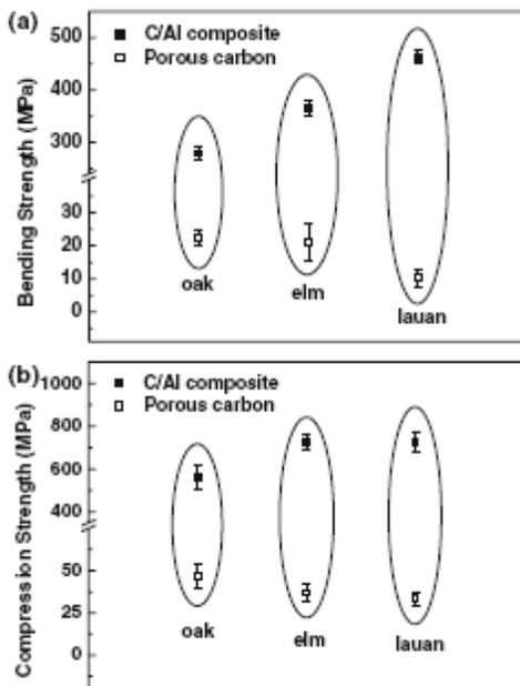
Figure 8. (a) Bending strength and (b) compression strength of porous carbon and C/Al composites [32].
