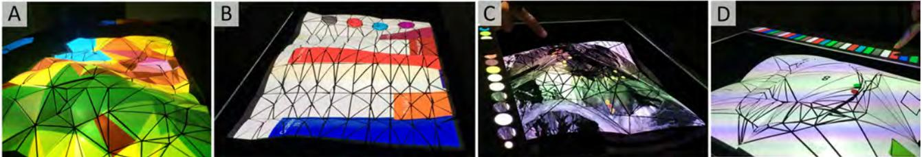
**Figure 1: Interactive shape-changing displays developed with PolySurface: A) a physical terrain model used for design session demos; B) physical bar-chart interface designed by P1; C) physical volcano modeling by P2; D) interactive physical display to model eye-tracking data by P3.**
