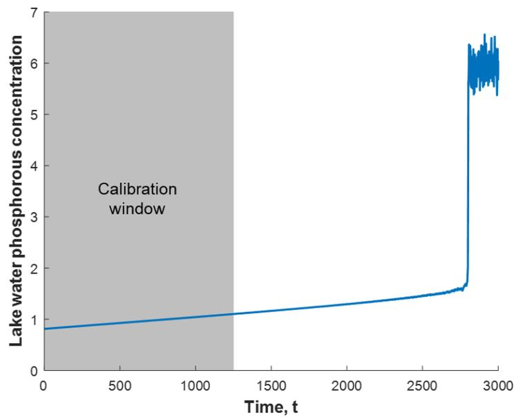
Figure 1: Simulated time series of the lake phosphorous concentration with linear ramping in phosphorous inflow. The system undergoes a saddle-node bifurcation at  $t \approx 2800$ . The grey region highlights the calibration window used to fit a 1D map to the delay coordinates.
