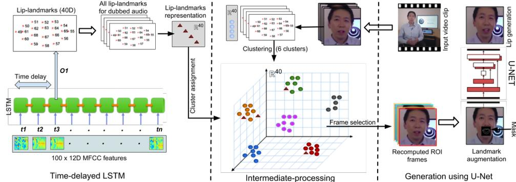
**Fig. 1.** Cross-language lip-sync: (left) Pipeline for training LSTM with Hindi speech and lip landmarks, (center) shows re-assignment of frames for each predicted lip-landmark using intermediate-processing step, (right) pipeline for inferring using U-Net on frames from English video.
