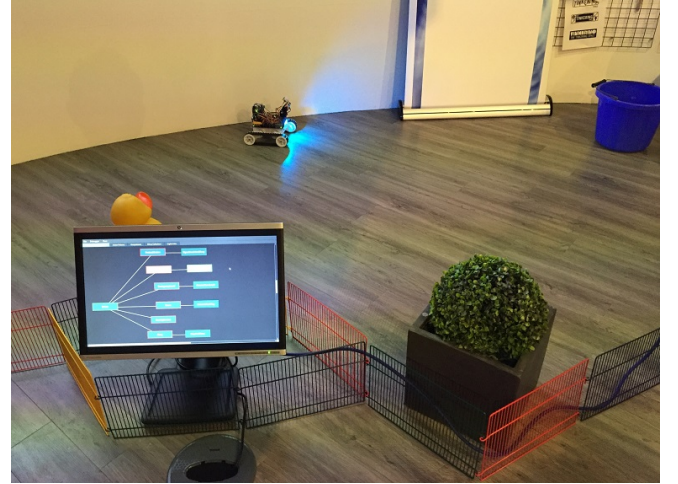
Fig. 5. The arrangement of the Directly Observed Robot experiment at At-Bristol. Obstacles visible include a yellow rubber duck and a blue bucket. The position and orientation of the transparency display is shown.
